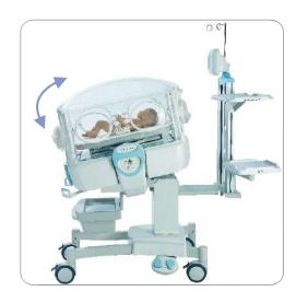
The canopy may be opened easily at the top or from the sides. The side walls open downwards using a unique mechanism that requires relatively small clearances at the sides of the incubator. This space-saving feature also means that it is easier to place the baby in the incubator or to remove it from within.
